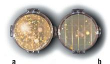
Agar plates incubated at 37 °C for 48 hours for air samples taken in a sealed room (Series 1): sample taken (a) prior to an 18-hour PowerZone-II run; (b) after a further one-hour operation of an air circulation fan.
